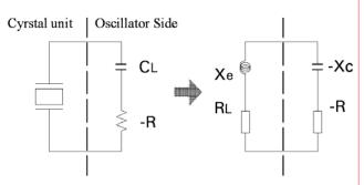
Equivalent circuit of Crystal unit and oscillator
